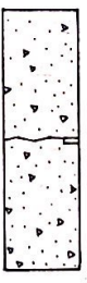
1/8" (3mm) PREFORMED OR METAL STRIP INSERTED WHEN CONCRETE IS PLACED; FINISH FLUSH WITH SURFACE
